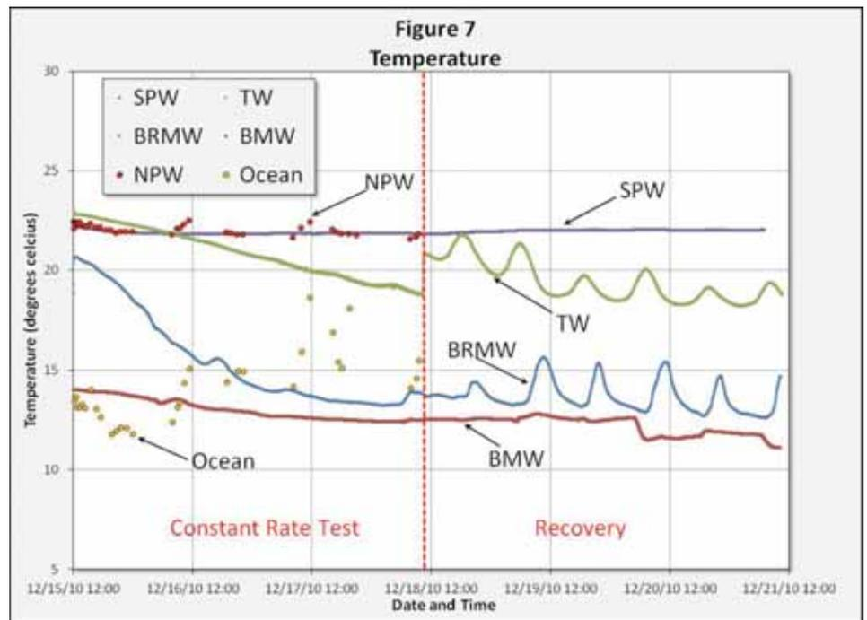
indicates that NPW was being redeveloped during the variable rate test. Based on the results of the variable rate test, it was determined that a pumping rate between 700 and 800 gpm could be sustained during the three-day constant rate test.
